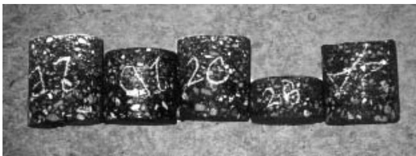
Comparison of cores taken across one lane show the extent of the deformation that has occurred.
