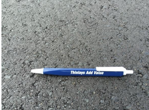
Figure 2: Thinlay Asphalt Concrete mat texture.
